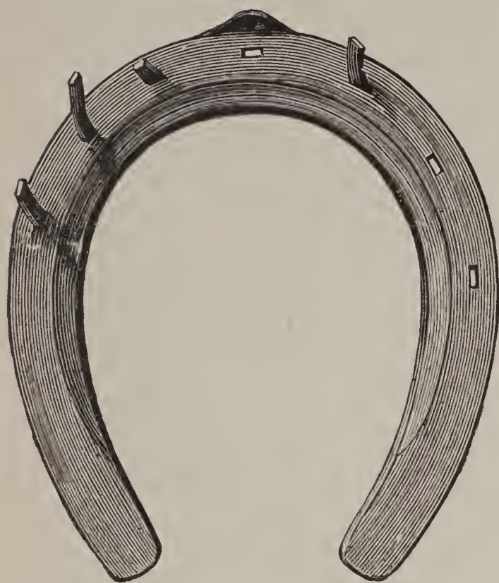
FIG. 202. — Model shoe-bearing surface.
