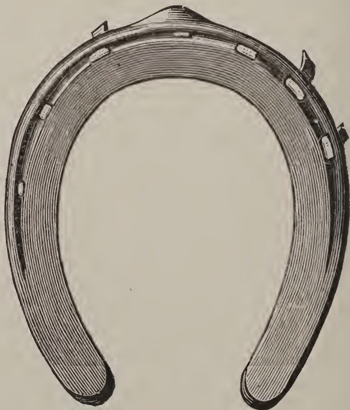
FIG. 203. — Model light drawing shoe.
